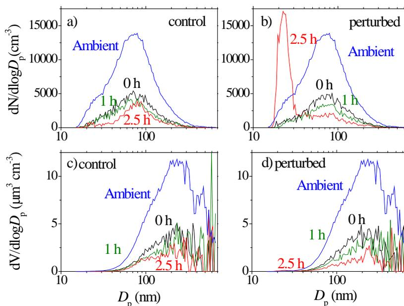
**Figure 2:** The SMPS-measured aerosol number and volume size distributions for the control and the perturbed chamber during Exp. 1.
