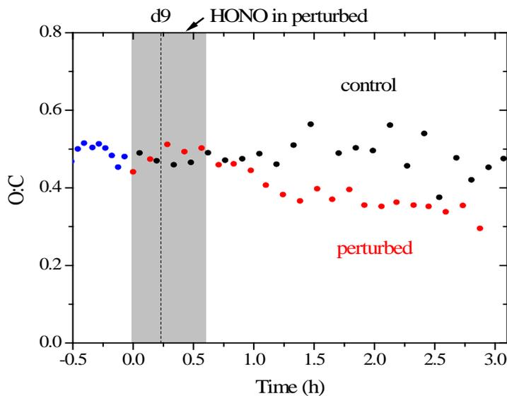
**Figure 3:** The atomic oxygen to carbon ratio (O:C) evolution of the AMS-measured organics during Exp. 1. At time zero, the instruments switched from measuring ambient (blue symbols) to the chambers. Butanol-d9 was added to both chambers at  $t=0.25$  h. At  $t=0.4$  h, HONO was added only to the perturbed chamber to produce OH under UV illumination. The shaded area indicates that the chambers were dark.
